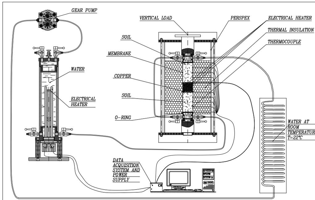
Figure 1. Test device
