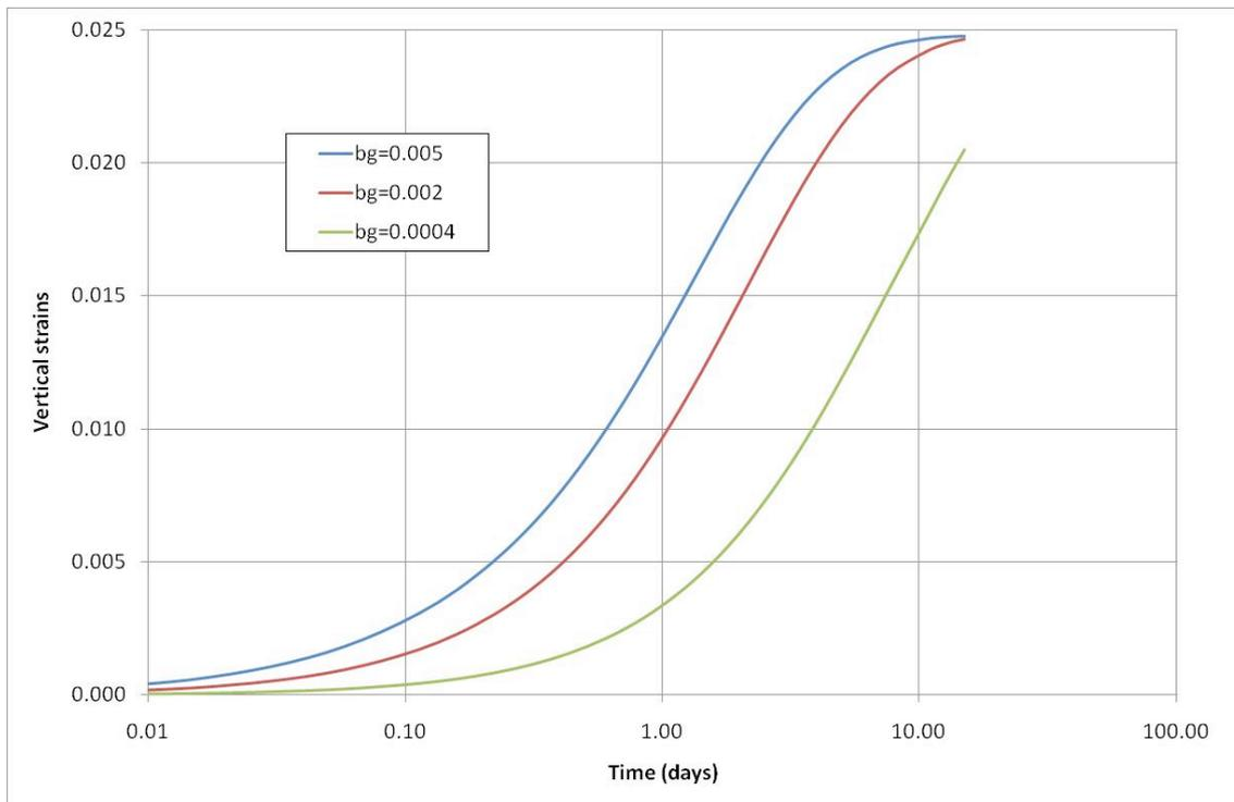
Figure 1. Vertical strains in suction controlled oedometer test
